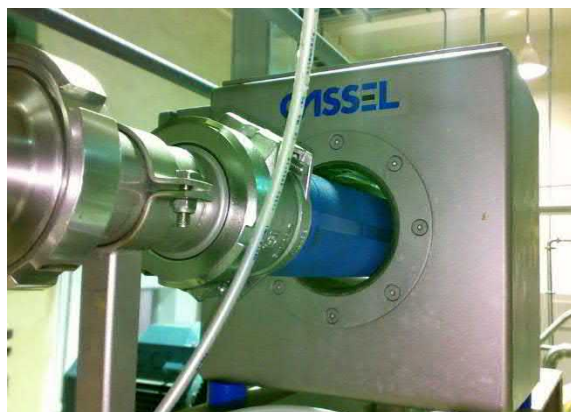
The pressure hose guarantees stability even at pressures up to 16 bar. For higher pressure up to 40 bar, pipe sections made of POM are used.
