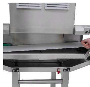
Release the conveyor belt.
