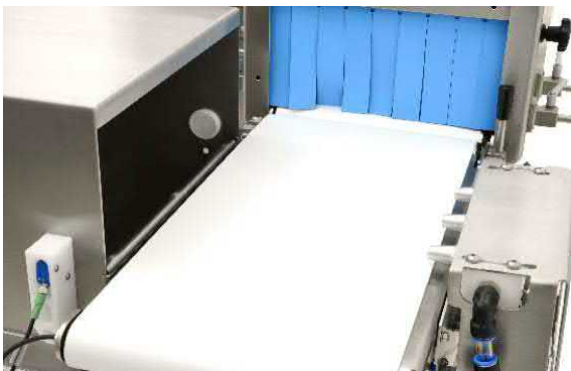
XRAY SHARK® XD38 with air pressure reject system.
