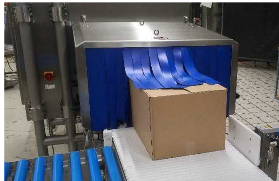
XRAY SHARK® XD47-H1 for package products in cardboard boxes.
